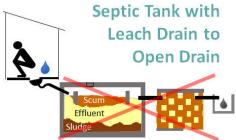
Figure 21: Septic tank with a leach drain discharging to the open drain
