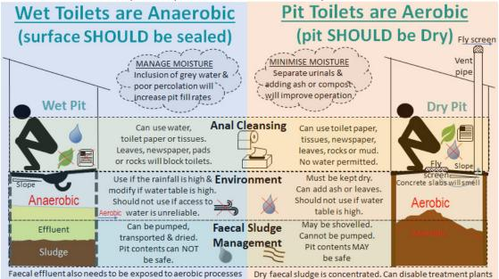
Figure 26: Aerobic versus anaerobic technology options
