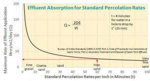
Figure 20: Effluent absorption for standard percolation rates
