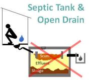
Figure 18: Unsanitary Septic Tank Design
