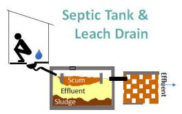
Figure 17: Sanitary Septic Tank Design
