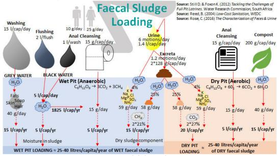
Figure 23: Faecal Sludge Loading Rates
