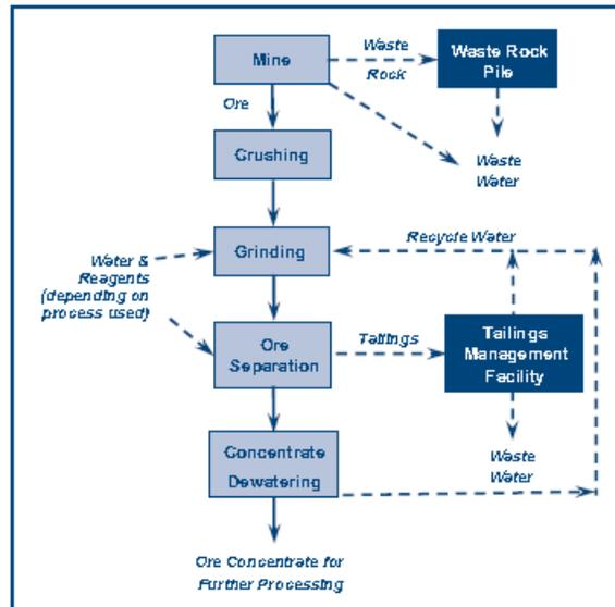
The concentration or separation process is conducted by physical and/or chemical methods, the objective of which is to produce an ore concentrate. The ore concentrate is sent to further processing, frequently offsite, to produce a marketable metal.
