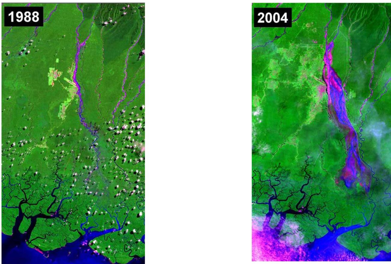
**Figure 16** Landsat photos of the expanding tailings deposition footprint in the Timika lowland area, from years as marked. Tailings deposits within the ADA visible as pink (dry tailings) and blue (waterlogged tailings). Dark black are standing water or cloud shadows. Cleared forest area visible as light green (from Paull et al 2006). (Source: WALHI 2006)
