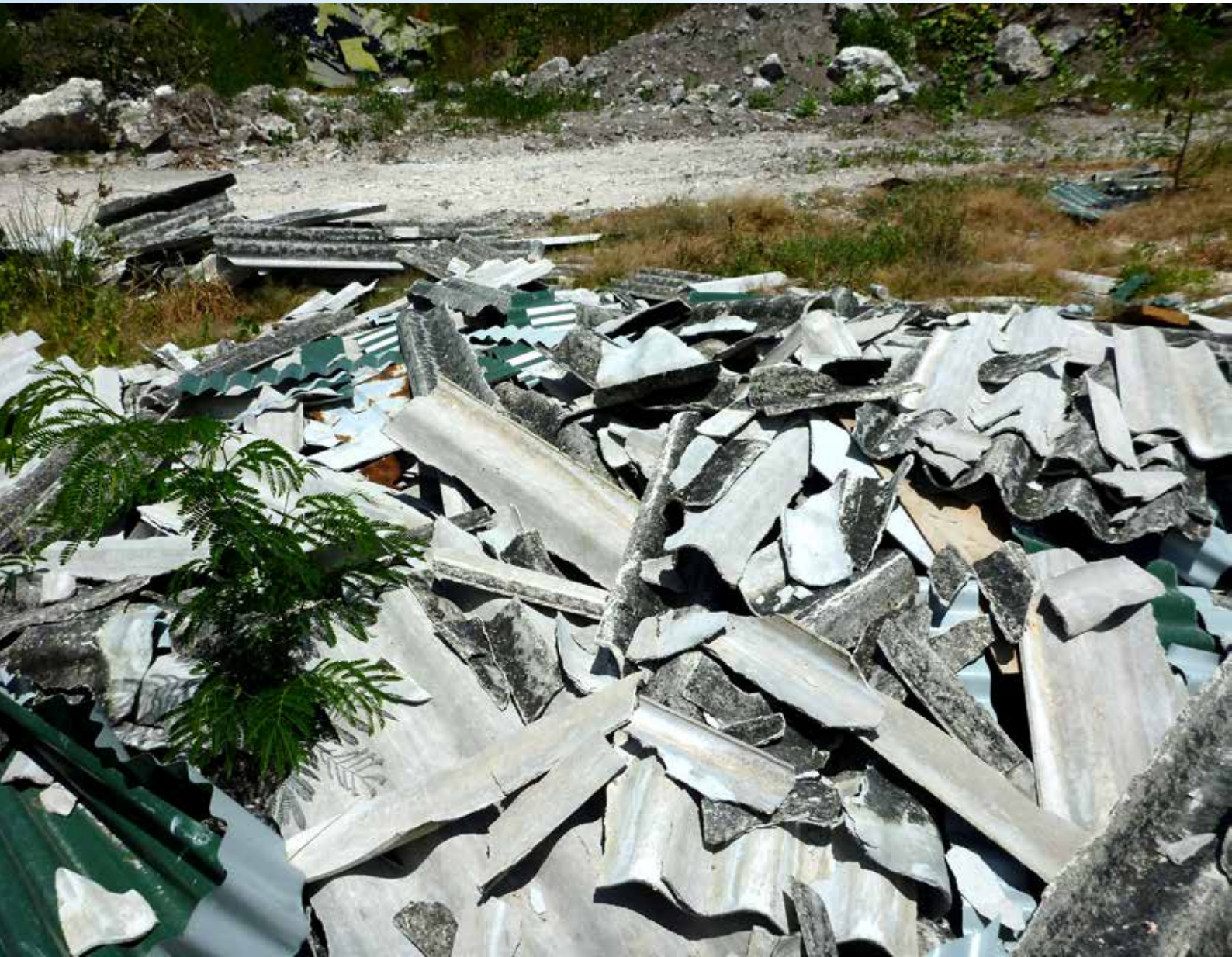
Asbestos cement sheeting is commonly found in the Pacific islands region. When damaged, these products can release dangerous asbestos fibres into the environment. Photo: © Esther Richards
