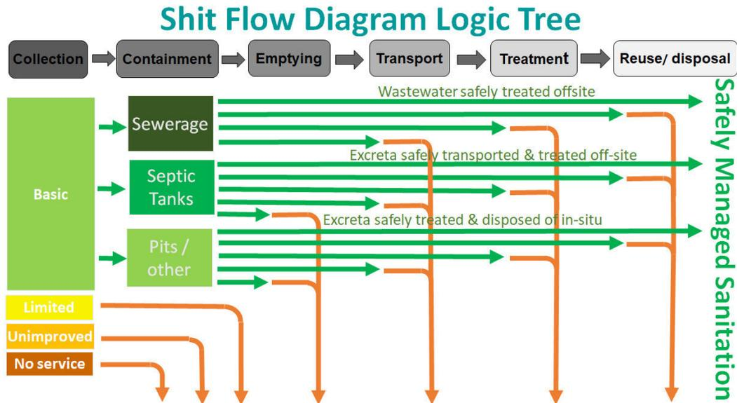
Figure 7: Shit Flow Diagram Logic Tree
