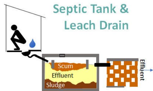
Figure 17: Sanitary Septic Tank Design
