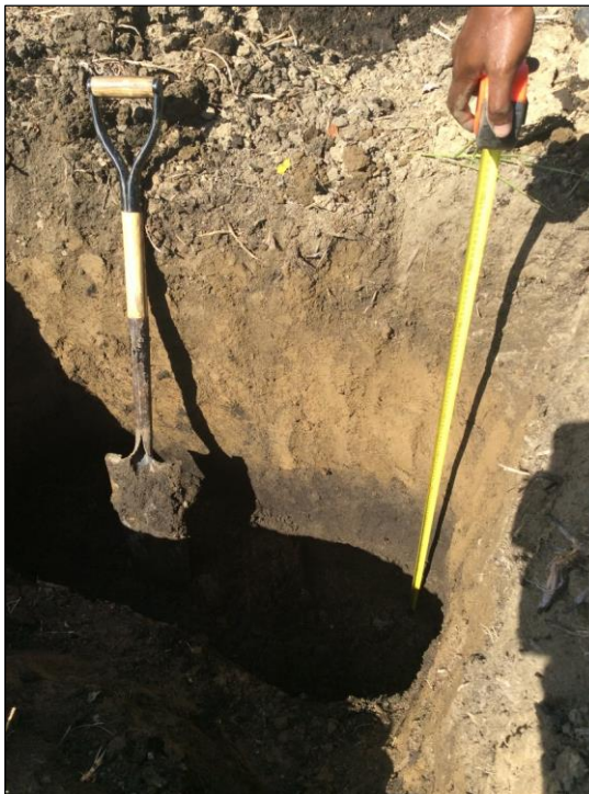
Plate 6.10 – Soil Pit at Ngararaf with Clay Loam Topsoil over Silt/Sand and Gravel
