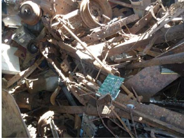
PCB mixed in with scrap steel for baling
