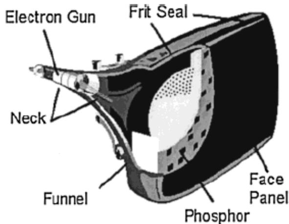
Figure 1: components of a typical CRT<sup>57</sup>
