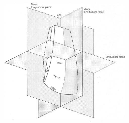
Fig.27 Trimetric projection of the main planes referred to in the text (In asymmetric axes, the major longitudinal plane does not pass through the edge; a fourth oblique plane equally bisects the bevels and passes through the edge: see Fig.28)
