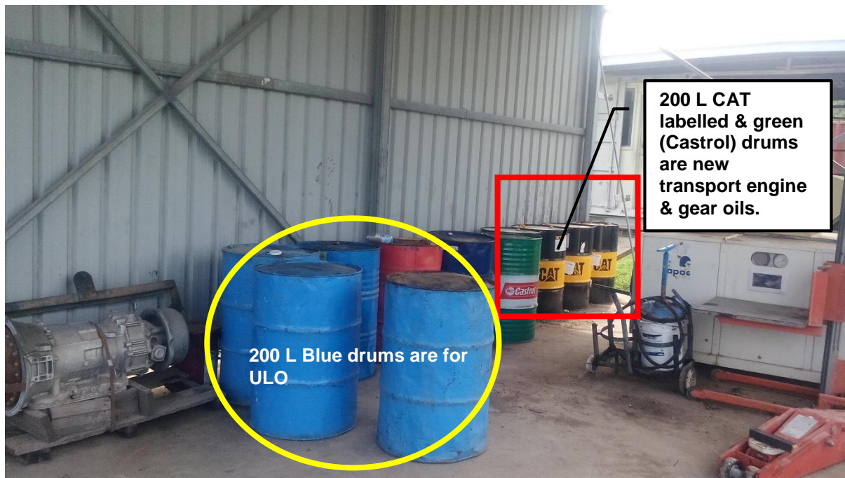
Figure 15. Example of a clean Oil and ULO storage area in a small workshop.
