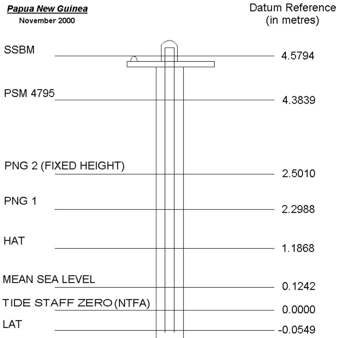
The word “datum” in relation to tide gauges and nautical charts means a reference level. Similarly, when you measure the height of a child, your datum is the floor on which the child stands.
