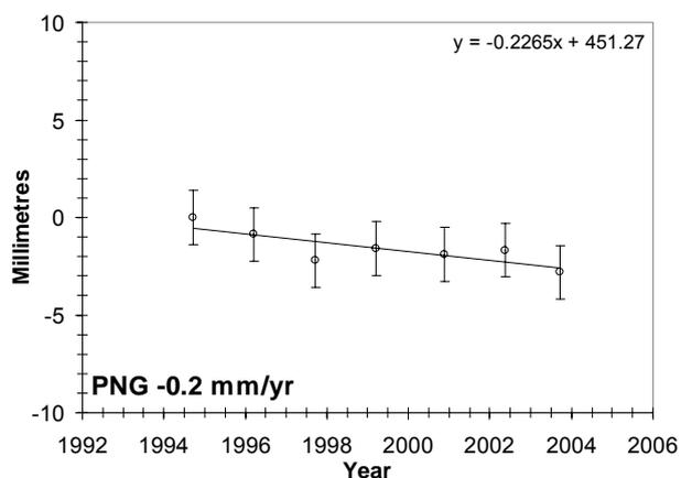
**Figure 19. Movement of the SEAFRAME Sensor relative to the Tide Gauge Bench Mark.**
