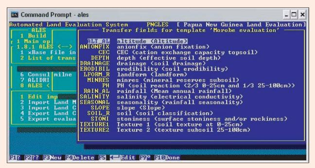
Figure 83: Assigning columns contained in the intersected PNGRIS table, shown in the left hand column in yellow, to the corresponding attribute contained in the PNGLES crop requirement database, shown in the right hand column in white.
