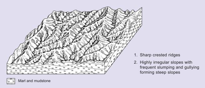
Mountains and hills with weak or no structural control on consolidated fine grained sedimentary rocks (Figure 38) have more uniform slopes and a coarser dissection pattern than on soft fine grained sedimentary rocks. Slopes are usually steep and partly influenced by rock structure, and valleys are V-shaped. Slumping is important and debris slides common particularly in areas of thinly laminated but relatively hard mudstones and shales.
