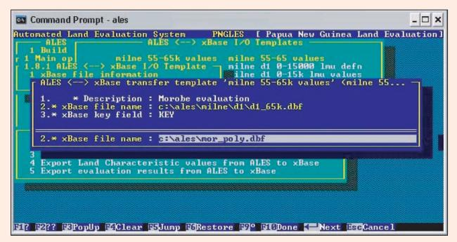
Figure 82: The file name of the table containing the climatic, topographic, and soil characteristics of the land being evaluated must be entered into PNGLES. In this example, the file is called 'mor\_poly.dbf'. This section of ALES is located by navigating to the 'ALES ⇒ xBASE' section of ALES.
