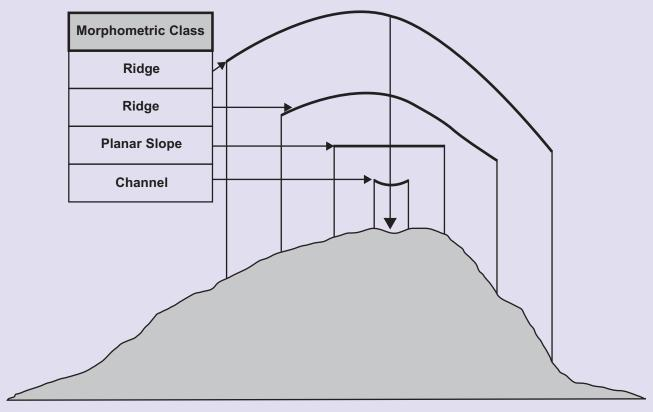
Figure 6: Topographic position (morphometric class) varies with the scale at which it is measured and also depends on the surrounding landscape. From: Fisher, Wood & Cheng (2003).
