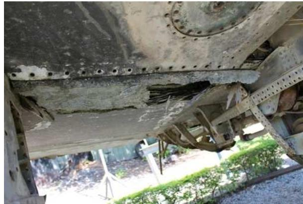
**Figure 2 Intergranular corrosion of a High strength alloy on a US Aircraft main spar cap.**
