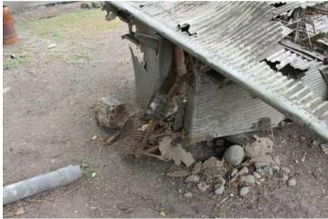
**Figure 6 Object imbedded in soil will suffer higher corrosion than an object clear of the soil.**
