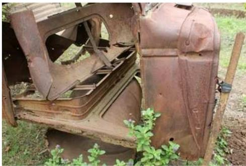
Figure 29 1940 Chevrolet 30cwt note lower parts missing due to corrosion from contact with moist dirt.
