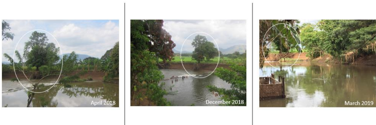
Figure 42. Three consecutive visits over 12 months illustrate the cohesive nature of the stream bank at Bomana pump station, where the circled tree remains insitu despite an extensive flood event in mid-February 2019.
