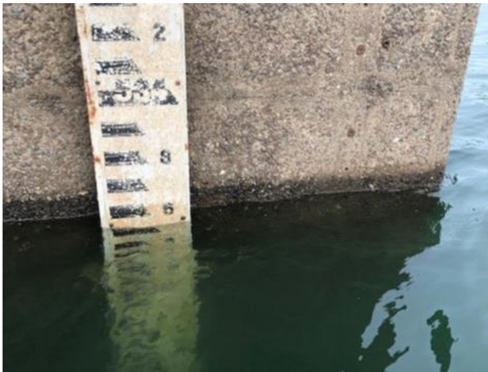
Figure 11 A snapshot of the reservoir water level of 533.5 m which did not change for the duration of the survey period.
